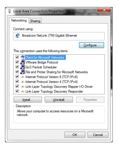
Now select "Internet Protocol Version 6 (TCP/IPv6)" and click "Properties", a new window appears allowing you to configure the IPv6 address, default gateway etc, this is shown on the below.
