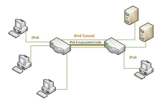
Tunneling provides a mechanism for transitioning an IPv4 network to IPv6 and/or maintaining interoperability between IPv4 and IPv6 networks.
